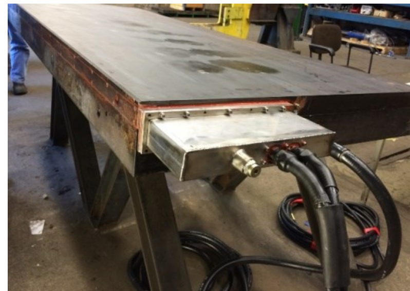
Example instrumented mold plate, with robust optical cable connections
